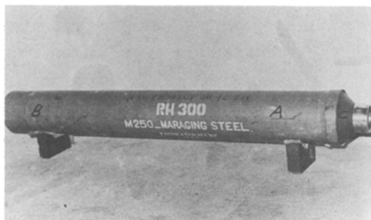
Figure 1 Maraging steel motor case (0.3 m in diameter, 2 m long, 0.0015 m thick). (A) Propulsion cylinder, (B) stub cylinder, (C) nozzle end.
